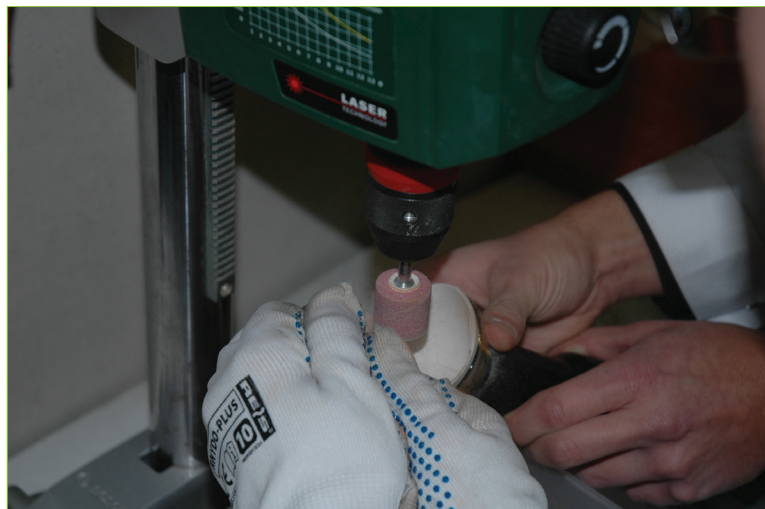
Fig. 7. Destructive tests – grinding of pottery for the purpose of its decomposition with hydrofluoric acid. Photo A. Michałowski.
