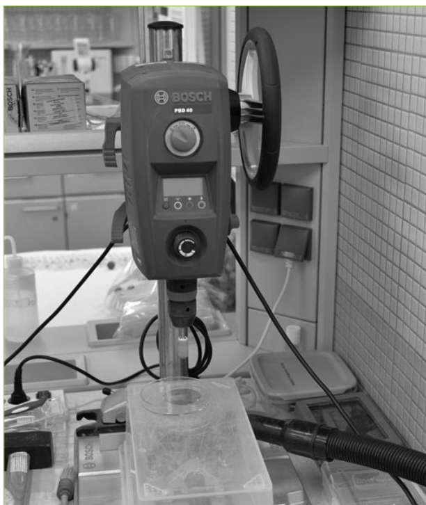
Fig. 3. The professional driller used to obtain the cylinders from pottery samples.
