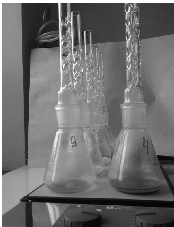
Fig. 6. Acid extraction of the cylinders surface or melted samples.
