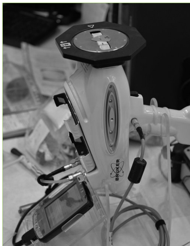
Fig. 2. The ED-XRF (energy dispersion X-ray fluorescence) Bruker Tracer III SD spectrometer used in analysis of the elemental composition of the pottery.
