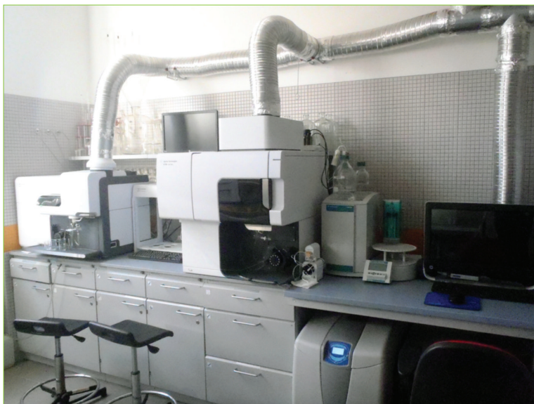
Fig. 8. Equipment used to determine the content of elements in solutions; left to right: a microwave induced plasma optical emission spectrometer, an inductively coupled plasma optical emission spectrometer, and an ion chromatograph. Photo P. Niedzielski.
