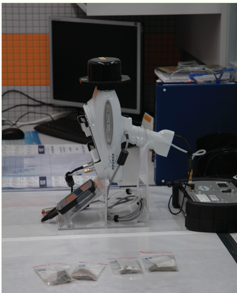
Fig. 5. The ED-XRF (energy dispersion X-ray fluorescence) Bruker Tracer III SD spectrometer used in the non-destructive tests performed on the pottery. Photo A. Michałowski.
