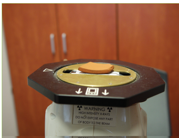
Fig. 2. The ceramic sample completely covering the outlet of the detector.
