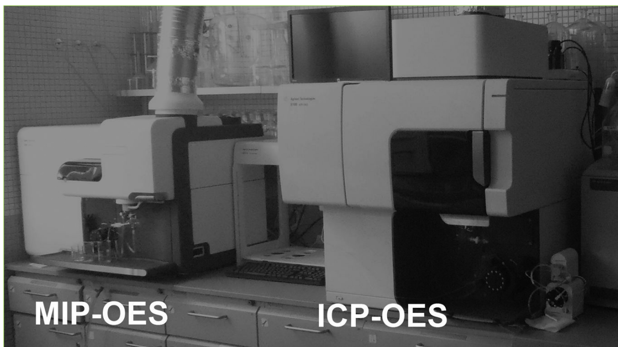
Fig.7. The plasma based optical emission spectrometers used for analysis of the extracts of the samples.
