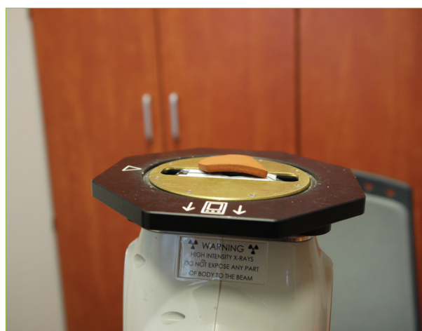
Fig. 3. The curvature of the ceramic sherd may have influence on the chemical results.
