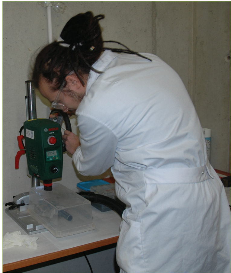
Fig. 6. Destructive tests – preparation of pottery material cores which, once the sides and one of the ends are protected with a chemically neutral varnish, will be subject to extraction with hydrochloric acid. Photo A. Michałowski.
