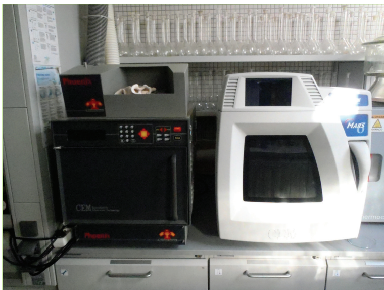
Fig. 9. Devices used on the project to prepare comparative samples of pottery and clay; left to right: a microwave oven and a microwave mineralization/digestion system. Photo P. Niedzielski.
